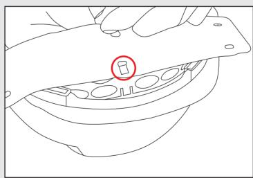
1. Remove the old sweatband from your EVO® safety hard hat 2. Place the holes from one side of the band over the tabs on the outside of the hard hat's suspension.
