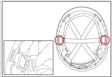
4. Now take the extra strap, thread the first clip between the suspension and the hard hat and click back down. Repeat this for the final clip, making sure that the strap is above the 2 diagonal straps already in place.
