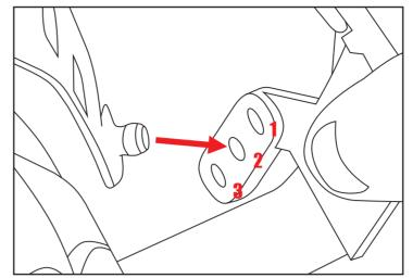
3. Then relocate the arm into 1 of 3 receivers. Repeat this process at all 4 adjustment points.
