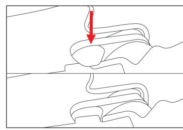
4. Push the spec down until the clips on the spec arm clip under the notches on the front webbing clips.
