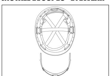
1. Lay the Evolution Deluxe hard hat and spec out like this. 2. The pins on the spec arms go into the sockets closest to 3. Once both pins are connected, slide the spec into the
